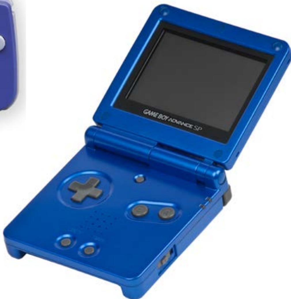
screen in the top. Internally it was similar to the first model, but added a front light for the screen and a Lithium Ion rechargeable battery. With the light off, you could squeeze 18 hours out of the device, as well as a respectable 10 with the light on. A later revision in 2005 saw the screen changed to backlit
