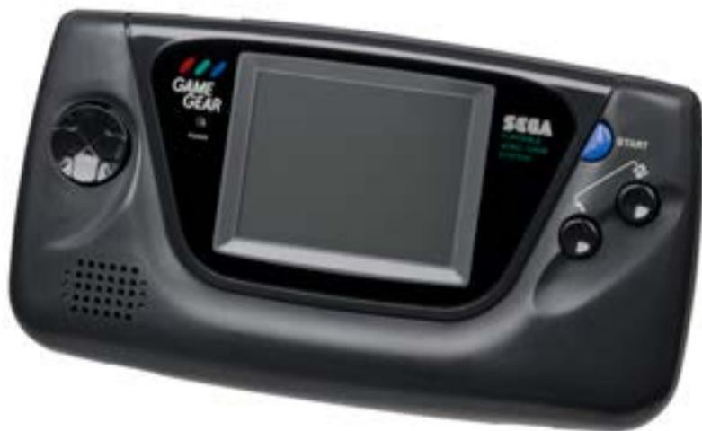
The Game Gear was the best-selling Game Boy competitor, shifting around 11 million units worldwide. It was essentially a portable Master System, although it took different shaped cartridges. Most Master System games can be played on the device with the use of an adapter. The high-end hardware and colour screen was attractive to many gamers compared to Nintendo's monochrome offering but like the Atari Lynx, its battery life was poor. As a result this harmed sales.
