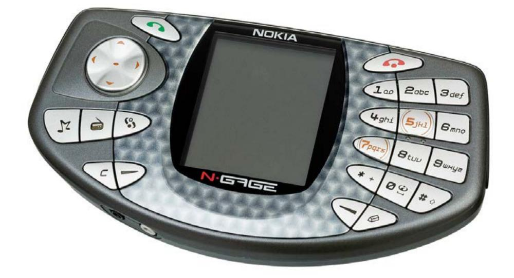
The device was not received well, with its unusual shape and speaker positioning on the side meaning it was awkward to use as a phone. As a game console it was equally awkward, with the battery needing to be removed to change cartridge and control buttons mixed in with the numeric keypad. A second model with a new design was released in 2004, called the N-Gage QD, but by this point
