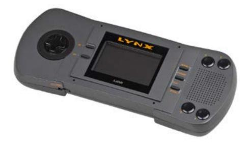
Arriving just three months after the North American release of the Game Boy, the Lynx was hugely more powerful than Nintendo's device. With a colour screen, two processors, and eight times the RAM, on paper, it was the much better system. Sadly a lack of support from developers led to a dearth of games. To make things worse, the extra power inside the system ate through batteries like Kevin James at a buffet and four AA batteries would get only four hours of gaming,
